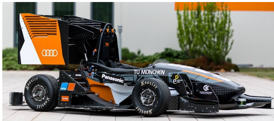
Figure 32: TU München's 2018 car featuring large diffusers built into their sidepod floors.
