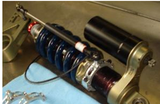
Figure 62: Shock potentiometer measures suspension travel.
