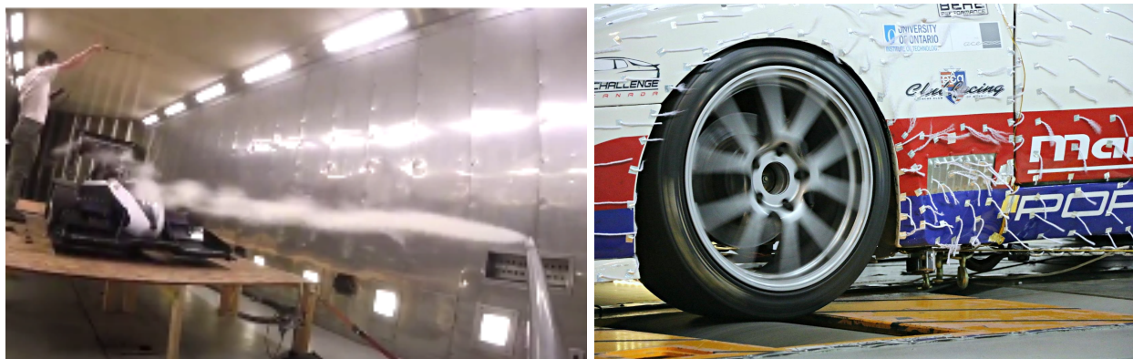
Figure 60: Flow visualization with smoke wand (left) and tufts (right) in wind tunnel.
