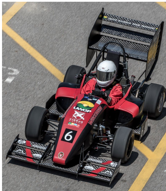
Figure 36: WR-217 at MIS. Note that the rear wing elements are trimmed down for the acceleration event.
