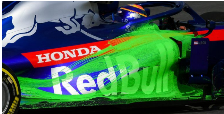
Figure 64: Flow Viz paint used on a Toro Rosso F1 car.
