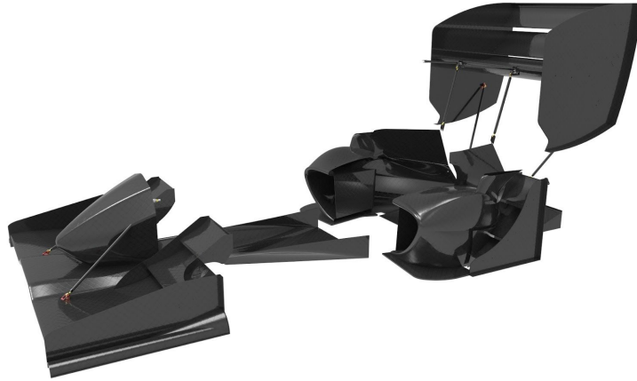
Figure 35: Render of WR-216 aero package. Note the underbody and side geometry. You can just see the diffuser peeking out the back.
