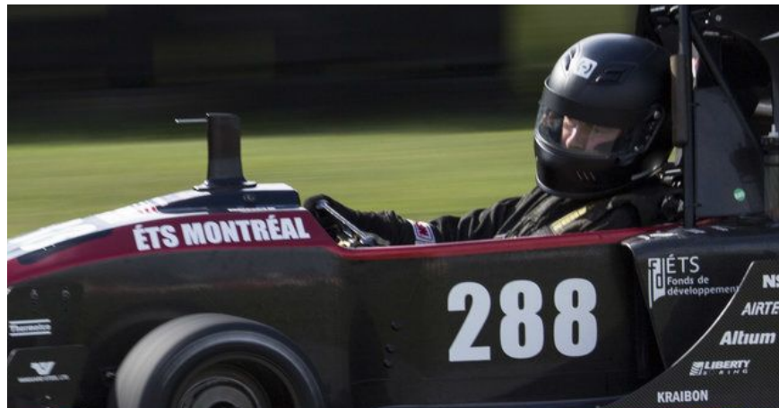
Figure 63: Pitot tube on ETS's car. Some FSAE cars have permanent pitot tubes used for active aero control.
