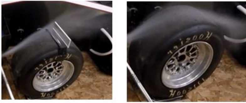
Figure 56: Simulating rotating wheel in wind tunnel with angle iron.
