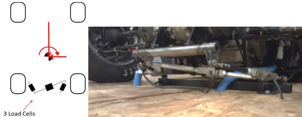
Figure 59: Wind tunnel load cell setup.
