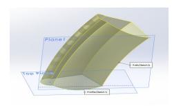
geometry. In the case of the picture to the right, the example sketch I created is being swept along a spline in another sketch.
