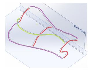
The red curves are the profiles, they show what a section of the surface would be in their plane. They are used as a start and end point, they also can be midpoints but
