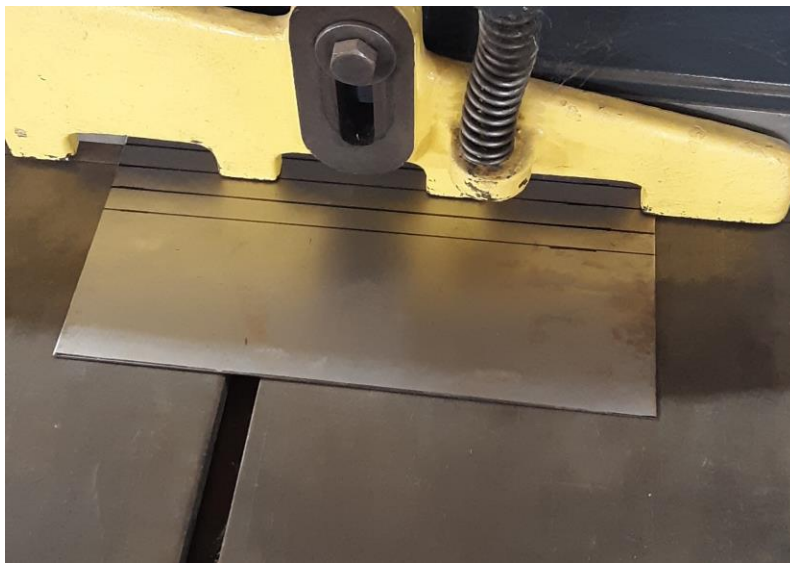
Figure 45. 0.06 Inch Steel Tabs Being Cut with Shear
