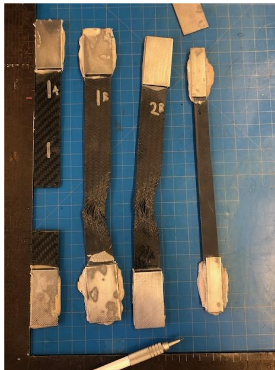
Figure 56: Failure of Selected Samples
