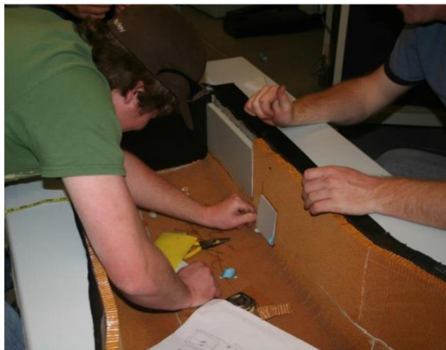
Figure 11. The 2015 Chassis Senior Project Team Inserting Balsa Reinforcements Into the Chassis.
