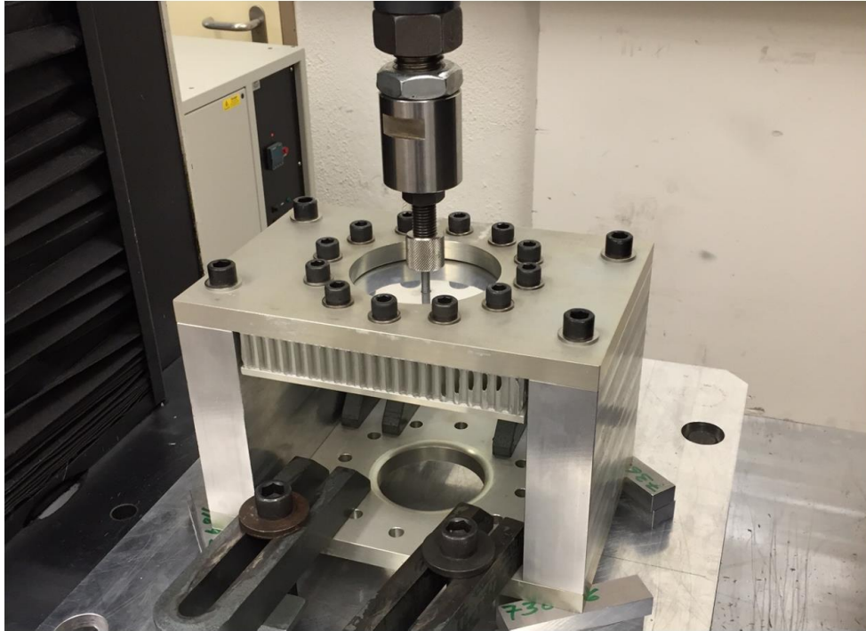
Figure 40. Testing Setup of a Hardpoint Pull-Out Test
