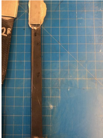
Figure 57: Failure of T700 Sample
