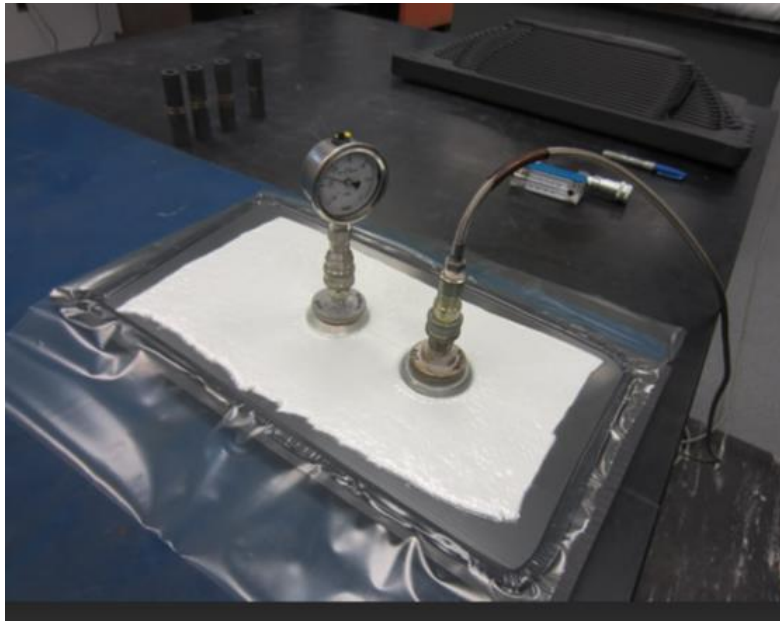
Figure 43. Sandwich Panel Prepared for Curing in a Vacuum Bag
