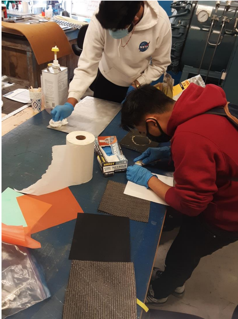
Figure 46: Cleaning the Vacuum Lay-up sheet and Removing Adhesive Lining
