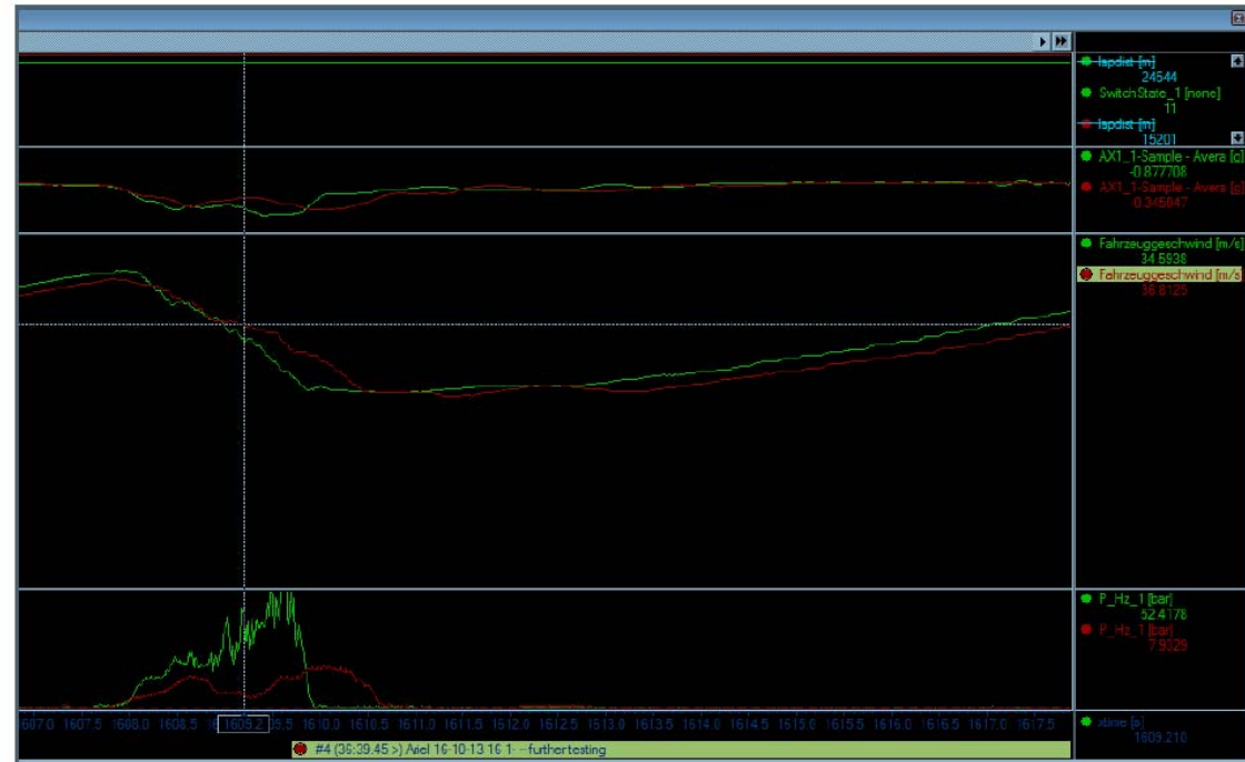
Fig 1 – ABS off (red) and ABS on (green) showing deceleration gains over rough surfaces.
