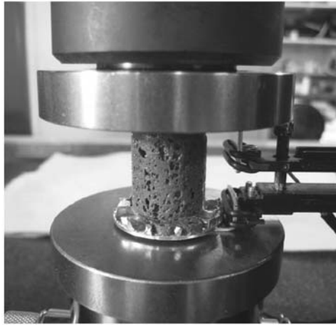
Figure 14. Compressive test of Redux 219/2-NA adhesive foam.
