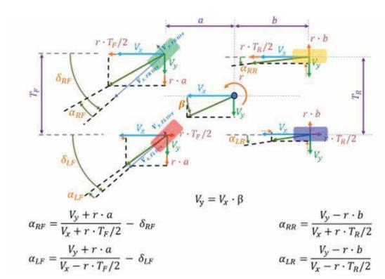
Figure 3: Tyre slip angle calculation
