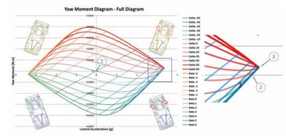
Figure 4: Yaw moment diagram at constant speed with CG slip angle and steering isolines
