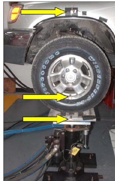
Figure 2. Placement of accelerometers
